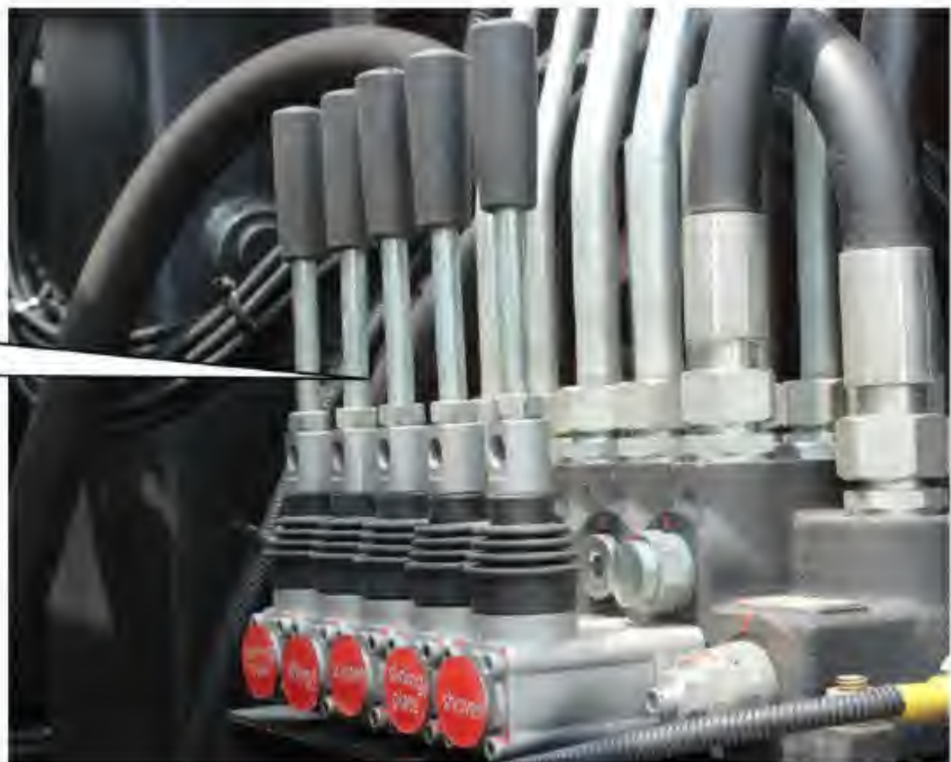
Hydraulic Control Joysticks (At drive side)
