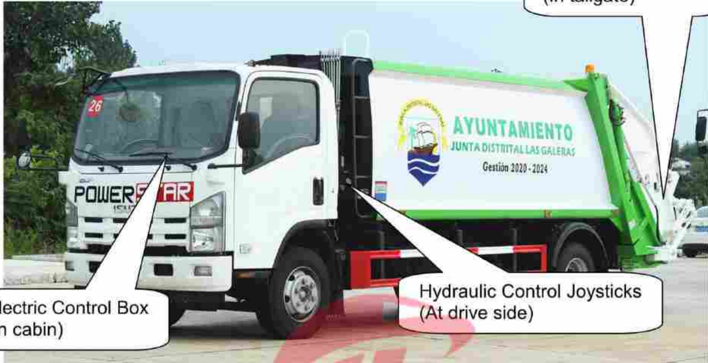
Front View: Hydraulic control system
